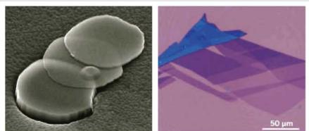
**THICK AND THIN** Multilayer graphite crystallites (gray, 2  $\mu$ m in diameter; thinnest is 30 atomic layers) can be thinned by successive peeling until they are reduced to a few, two, or just one (ranging from dark purple to nearly transparent regions) layer of graphene.
